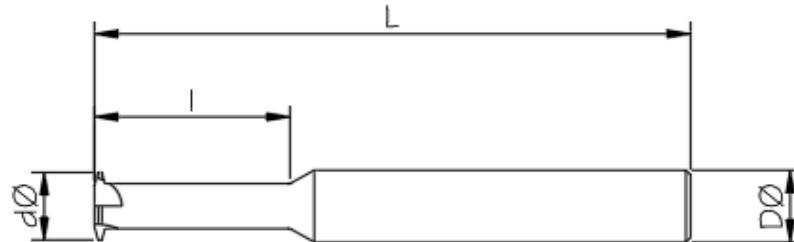
Designed to be used from the bottom to the top of thread, producing one full pitch every revolution of the thread.
